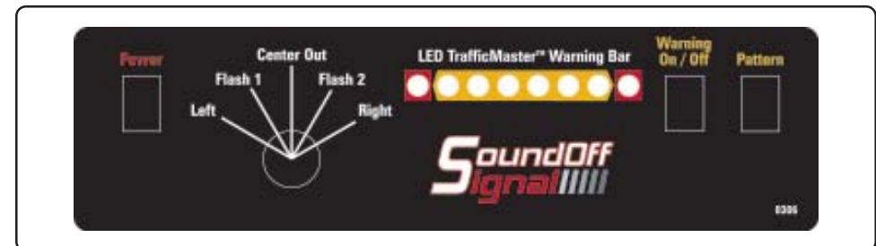
Figure 6. Control Module Faceplate
