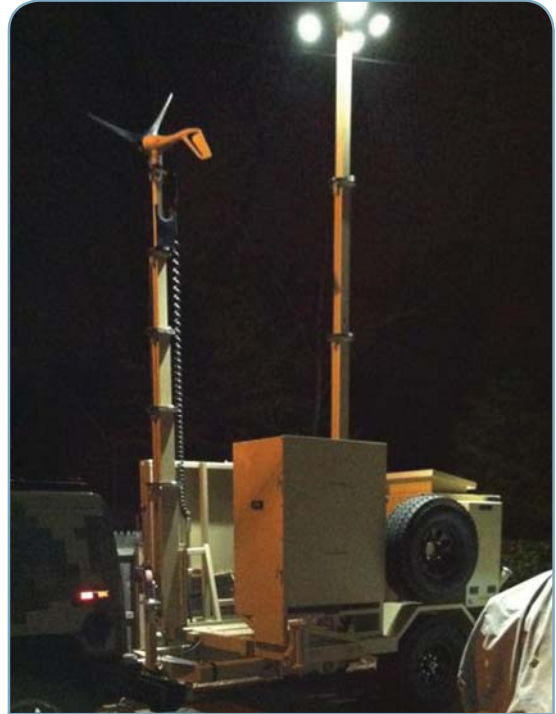
Lights mounted on mast at 21' off the ground provide bright white light & plenty of illumination for work area.
