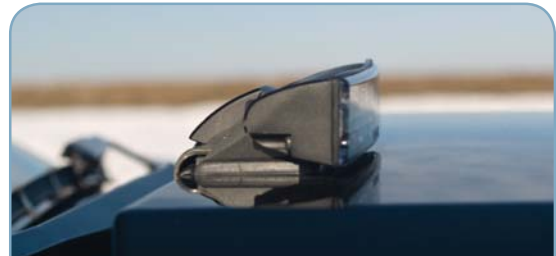
Single Light in Black Edge Mounted to the hood on a Ford Mustang police vehicle.
