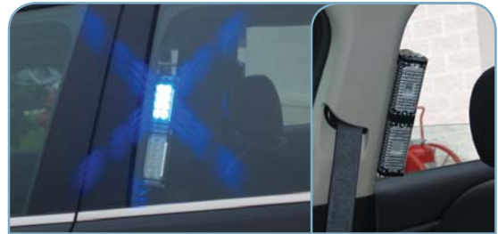
Predator 2™ Dual lights mounted in the interior on an undercover Chevrolet Caprice offer discrete side warning.
