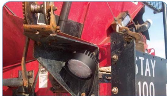
500 Lumen work light shown mounted on the rear of a DOT salt truck provides light in an otherwise dark area.
