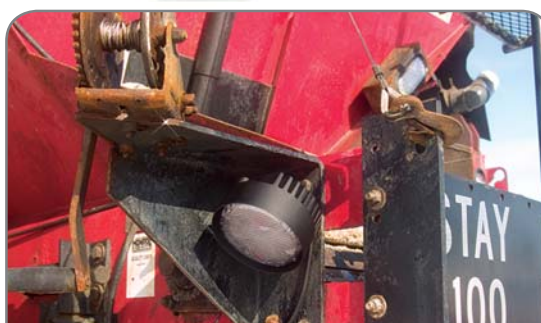
500 Lumen work light shown mounted on the rear of a DOT salt truck provides light in an otherwise dark area.
