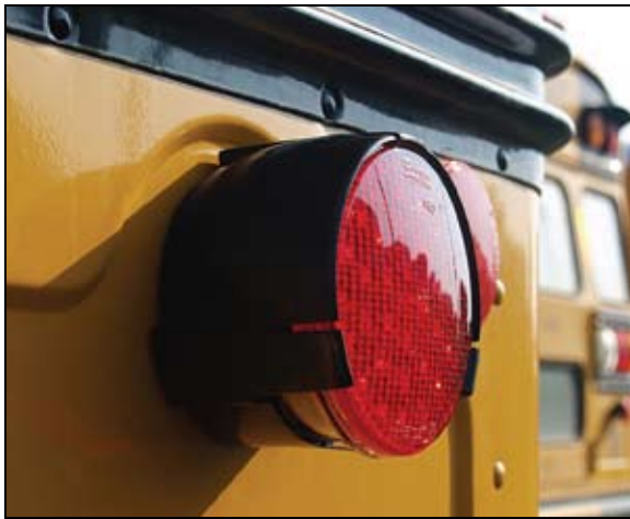
R4 RD Series STT/License Plate light mounted above the license plate area of a school bus.
